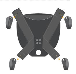
3. Attach the flat feet to the FLS cart using a flathead screwdriver
